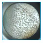
4. In a matter of seconds, your macro crystals will be crushed into micro crystals. Remove and set the Crystal Crusher aside. Seal the experiment using HR4-508, 0.75 inch wide Crystal Clear Mini Sealing Tape.
