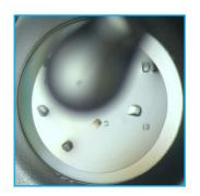
2. Working quickly, to minimize evaporation from the drop, position the Crystal Crusher above the drop well, the hemispherical end positioned down towards the drop.
