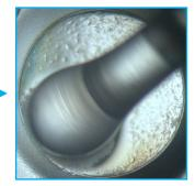
3. Lower the Crystal Crusher into the drop and begin crushing the macro crystals into micro crystals with a gentle up and down motion throughout the entire drop. Keep the Crystal Crusher in the drop, this is no time to get silly and splash or spread the drop you brute.
