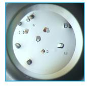
1. Position the crystallization plate and drop well containing the crystals to be crushed under the microscope. Using the HR4-124 X-Acto Gripster Knife, cut the film around the well and remove the film using a forcep.
